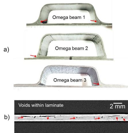
**Figure 1.** Photographic evidence of manufacture induced defects: a) Diamond arrows pointing to resin rich noodles; and b) normal arrows pointing to voids within laminate.
