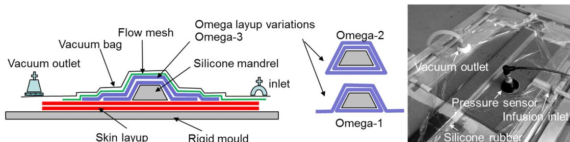
**Figure 2.** Sketch (Left) and actual setup (Right) of vacuum assisted resin transfer moulding for manufacturing Omega beam 1, 2 and 3
