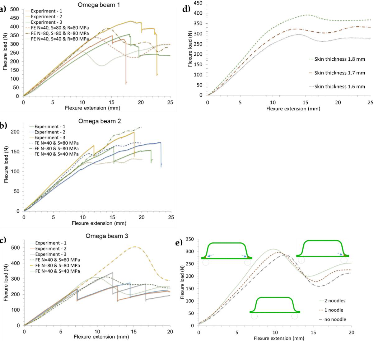
**Figure 3.** a, b, and c) Curves of flexure load vs flexure extension from experiment and FE prediction; d) Influence of skin thickness on the 4-point bending performance of Omega beam 1; e) Influence of resin rich noodles on the 4-point bending performance of Omega beam 3.
